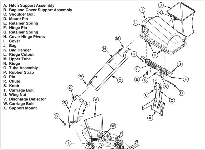
Figure 9. Normal Installation & Removal
